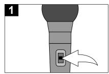
To turn the microphone on, slide the ON/OFF switch, located on the side of the microphone, to the ON position. To turn the microphone off, slide the ON/OFF switch to the OFF position. For the sound effect microphone, please refer to pages 15 and 16.
